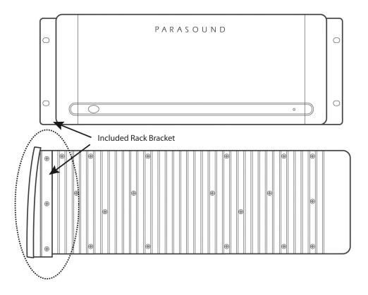
Note: Tighten each bolt just enough to keep the unit secure in the rack to avoid deforming the shoulder washers. Eliminating metal-to-metal contact reduces the likelihood of creating a ground loop that might introduce hum into your system.
